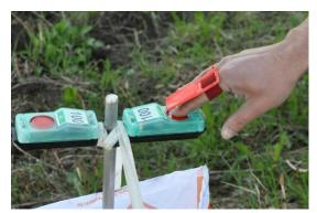
Press red button on the unit by finger that carries a card. Wait for acoustic and light feedback from the unit. A122 cards have on-board light feedback (10 flashing cycles within 5 sec. after punch)
